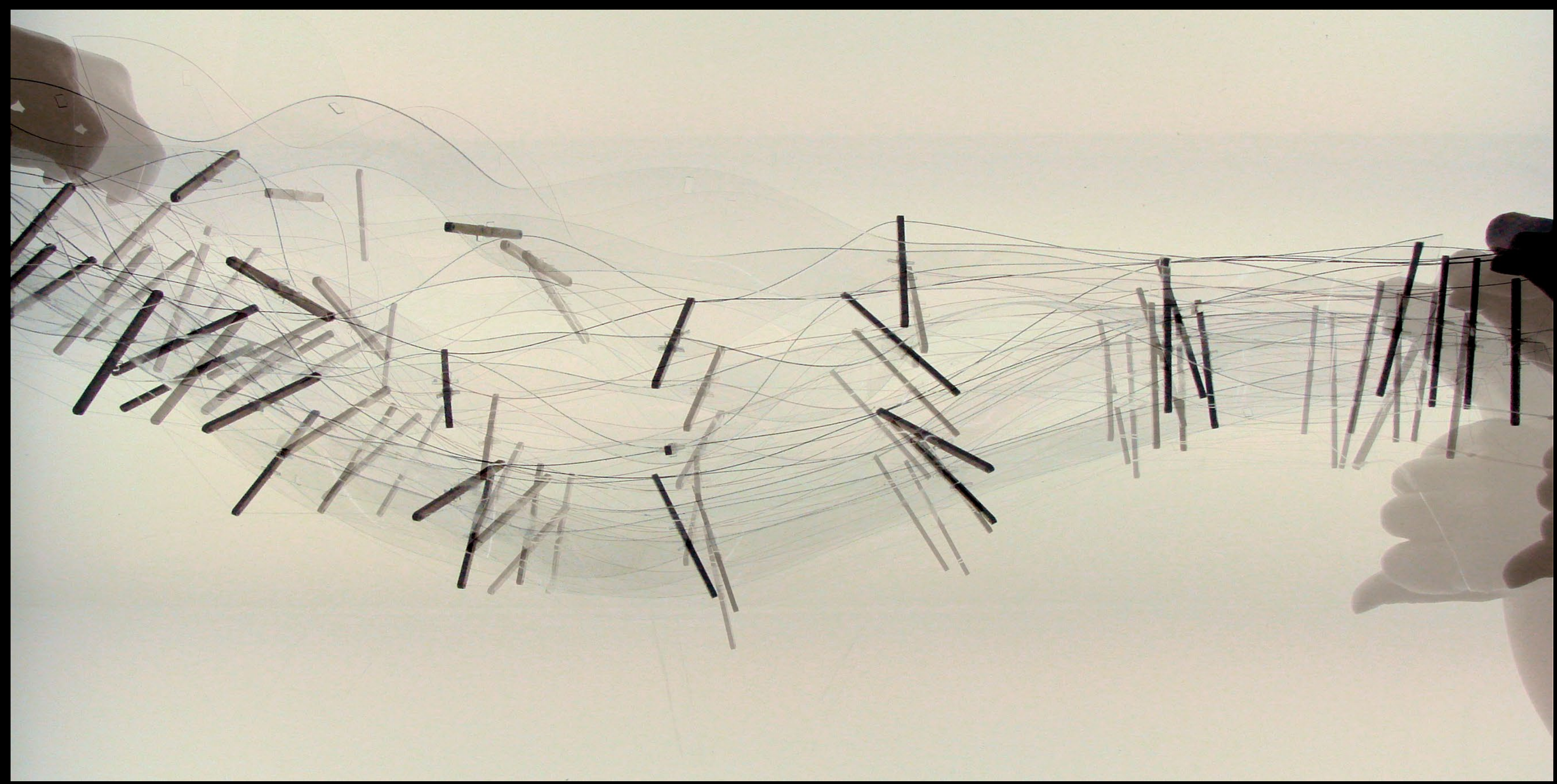
ELEVATION OVERLAY: THE MODEL EXPANDING AND CONTRACTING WITH THE USE OF TENSION TO OPEN AND CLOSE APERTURES
